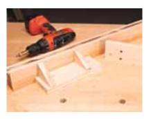
FENCE BRACES The fence is supported by two simple brackets screwed to the rear of the fence. The location of the triangular braces is important to the track orientation, so follow the diagrams carefully for location.
