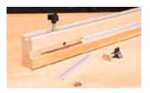
LAYING TRACKS Install the T-slot tracks in the grooves with flat head screws countersunk into the track. The braces are attached to the fence by screwing through the face groove prior to attaching the T-slot track.
