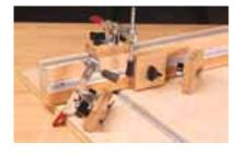
HOLD IT The hold-downs and stops are made from 3/4" hardwood. To make the guide to hold the stops square to the fence, cut a 1/16" x 1-1/8" rabbet on both sides of the inside face.
