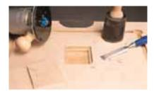
RABBET FOR THE INSERT After cutting the hole with a jigsaw, the opening is rabbeted using a bearing-piloted router bit. Then chisel the corners square and fit the replaceable center tightly into the rabbet. Make a couple extras.
